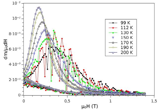
Figure 7. Differential susceptibility obtained from loops shown in Fig. 6. Discontinuities are observed on the ascending branch. Only the positive field side is shown.
