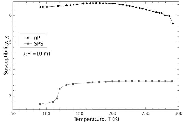
Figure 2. Susceptibility of magnetite in the form of nanoparticles (nP) and nanostructured ceramic sintered by means of SPS
