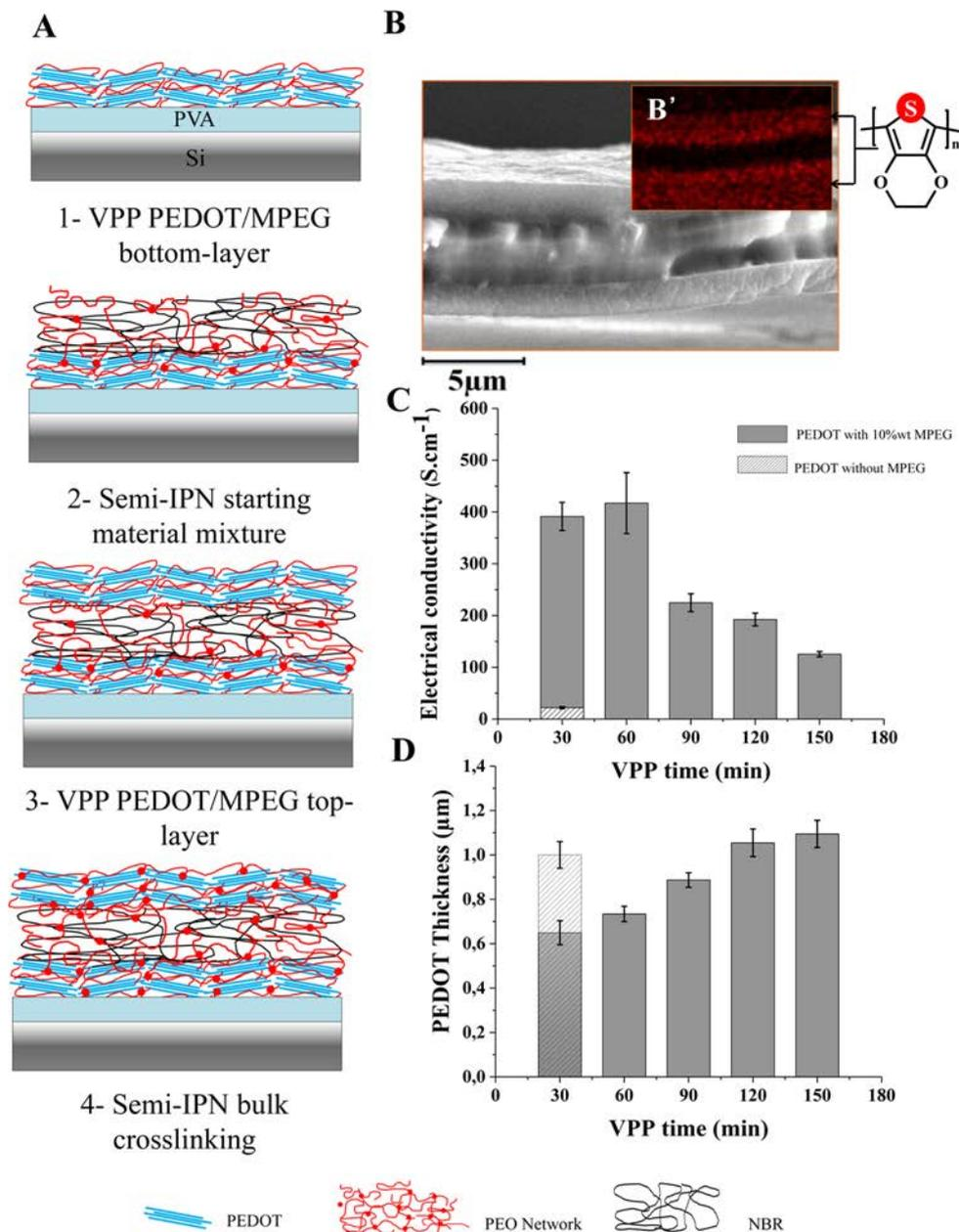
**Figure 2.** (A) On-substrate fabrication process of the PEO-NBR-PEDOT conducting semi-IPN. (B) SEM image of nonswollen trilayer structure and (B') corresponding EDS picture with sulfur atom cartography (red). (C) Influences of polymerization time on electrical conductivity and (D) on film thickness of PEDOT film synthesized in the presence of 10 wt % of MPEG.
