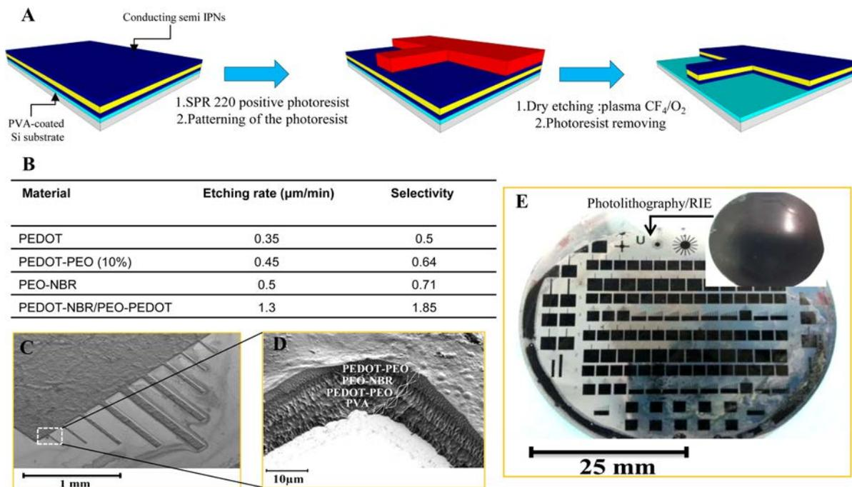
**Figure 3.** (A) Dry etching process of trilayer actuators on silicon substrate. (B) Etching rates and selectivity of PEDOT, PEDOT-PEO, PEO-NBR semi IPN, and PEDOT-PEO-NBR conducting semi IPNs in plasma of 90/10  $\text{O}_2/\text{CF}_4$  at 300 W and 200 mTorr. (C) SEM image of trilayer microstructures and (D) the corresponding zoom-in SEM image. (E) Image of the trilayer microstructures on PVA-coated 2 in. Si substrate. The inset show the trilayer coated substrate before microfabrication.
