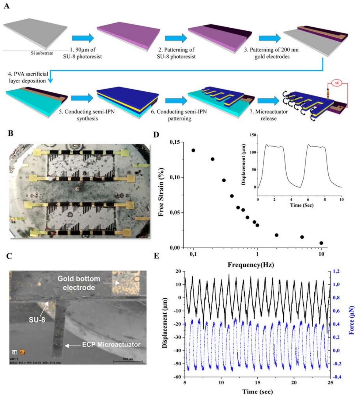
**Figure 4.** (A) Top-down fabrication process of trilayer microactuators on flexible substrate, (B) images of microactuators after batch microfabrication, (C) standalone microactuator on SU-8 substrate, (D) free strain as a function of frequency of the microactuator ( $Lwh$ :  $650\ \mu\text{m} \times 100\ \mu\text{m} \times 10\ \mu\text{m}$ ) under  $\pm 4\ \text{V}$  square wave potential, (E) tip displacement and output force versus time at 0.2 Hz.
