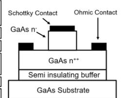
**Figure 2.** GaAs Schottky diode structure
