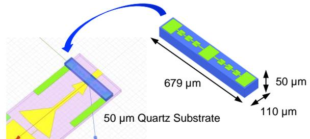
**Figure 1.** 3D model of 6 anodes doubler
