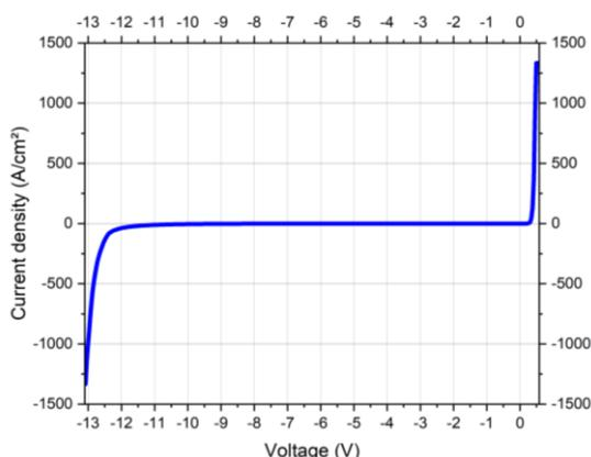
**Figure 4.** Typical 75 $\mu\text{m}^2$  anode IV characteristic
